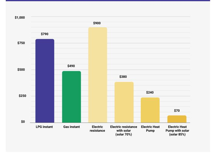
**Sources:** Rewiring Australia analysis. Residential Baseline Study 2021, heat pump COP 3.6, resistance tank 0.9, gas/LPG instant 0.95, gas/LPG tank 0.86. Electricity \$0.33kWh, gas \$0.14/kWh, LPG \$0.29/kWh, wood \$0.13/kWh. Solar \$855/kW financed at 5.5% over 30 years with replacement inverter.
